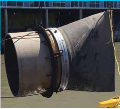
Detail of the ProFlex™ Flanged/Slip-On Slope Bottom Check Valve; Style 731
