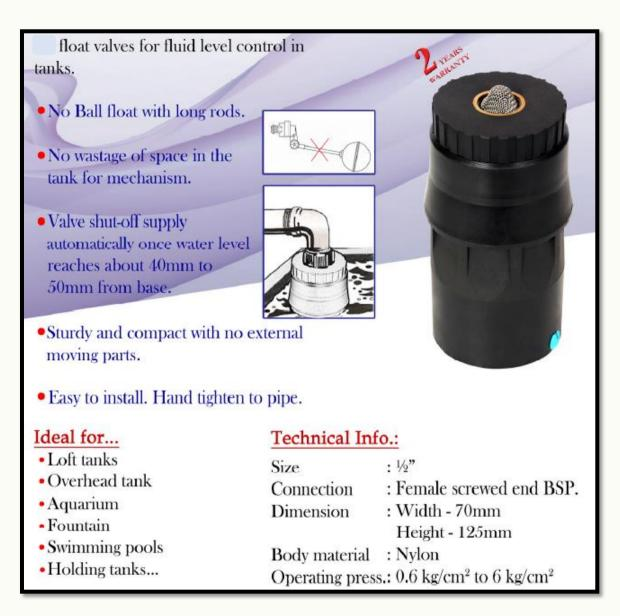
A new generation tank level controller. It is the most compact float valve which automatically turns off the water supply once the tank is filled up. The unique diaphragm of the Float uses the water pressure itself to stop the water flow in the tank. As the water level in tank reaches to a certain level (of about 30-50 mm) above base of the Float) the float inside rises, activates the diaphragm, and shuts off the water supply completely.
